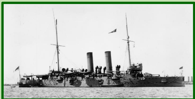
12. HMS Hawke - Edgar Class Cruiser, built Chatham Dockyard, Launched 1891, 7,770 tons.
